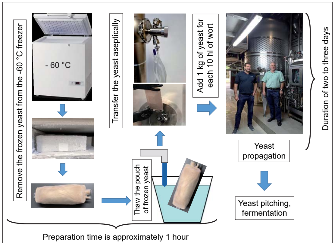
Fig. 2 Instructions for use (removal from the freezer, thawing, aseptic transfer, propagation) of the SmartBew™ Lager – TUM 34/70 bottom-fermenting frozen yeast product, spanning the period until yeast propagation begins through subsequent pitching to initiate fermentation (total time until the yeast is ready to pitch: two to three days, preparation time of 1 h)
